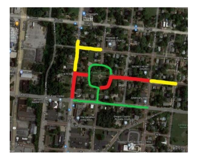
Turner Tract Area: Danforth Street will be closing in the next week or two to all thru traffic to allow for sewer installation work. The alley south of McKinley east of Lincoln is back open to traffic, with pavement restoration happening as weather permits. Douglas Street, between State and Lincoln Streets is closed for sewer installation work.
