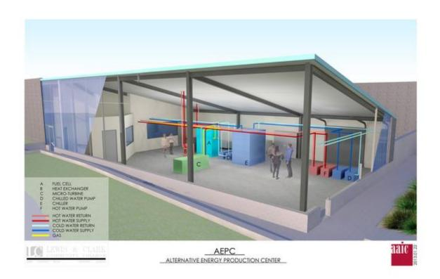
The fuel cell, expected to be installed in November 2013, will be placed in the Trimpe Building as part of the planned renovations for the building that will take place over the next 18 months. The fuel cell will be the first alternative energy source added to the site that will soon be known as the Alternative Energy Production Center (AEPC) at Lewis and Clark.
